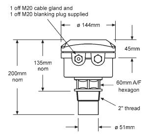
The transmitter is mounted using the 2" thread provided. An optional mounting bracket kit is available on request. MSP-BRK2 (2" BSPT) or MSP-BRK3 (2" NPT).
